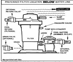
NOTE: ANSI/NSPI-4 Article V. standard for above-ground and on-ground pools, advises that components such as the filtration system, pump and heater be positioned so as to prevent their being used as a mea access to the pool by young children.
